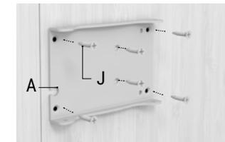
**4.** Attach the base plate (A) to the door using the screws (J) supplied.
