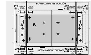
**2A.** Place the installation template in the chosen position and, on the door, use a pen to mark the holes corresponding to the body of the lock (shown as letter B on the template) and to the bolt housing (shown as letters A or C, depending on which side it is installed).
