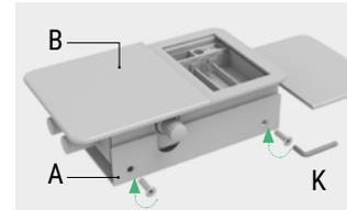
**1.** Separate the base plate (A) from the body of the lock (B) by removing the screws with the Allen key supplied.
